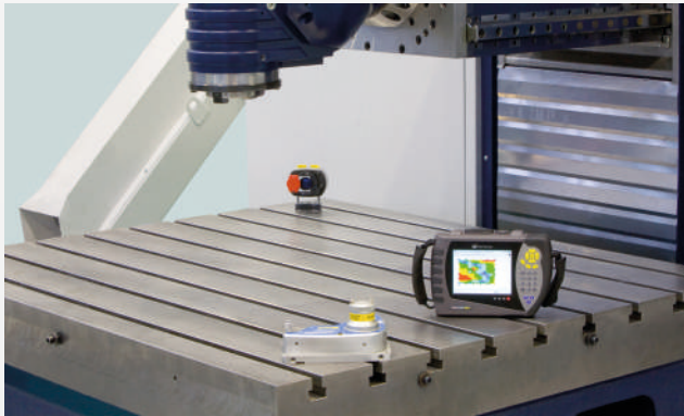
Flatness measurement of a machine tool table with LEVALIGN® Ultra
