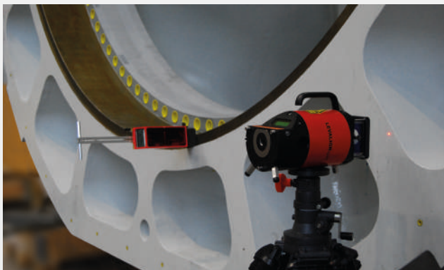
Flatness measurement of a wind turbine hub flange with LEVALIGN® Expert
